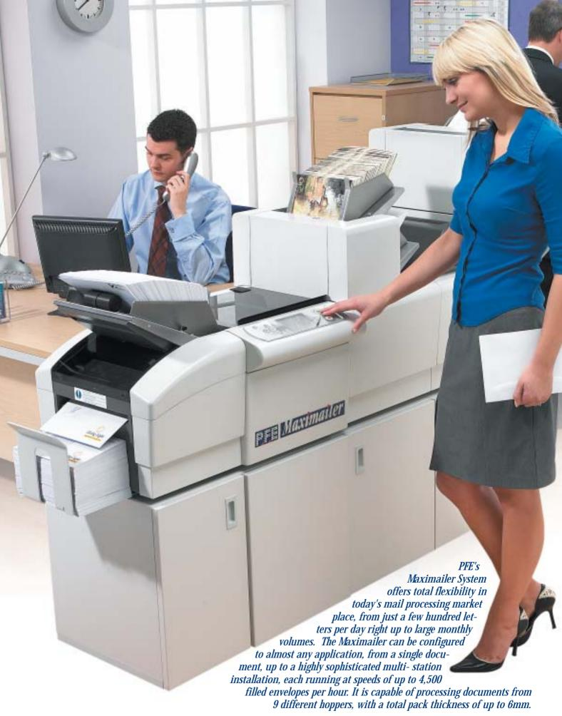
The graphical display and operating software guide you simply through creating and running the most complex of applications, even allowing the document containing the address to be in any hopper.
